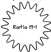
(b) Spot-wheel patterns obtained by inserting high frequency at point A to modulate light intensity
